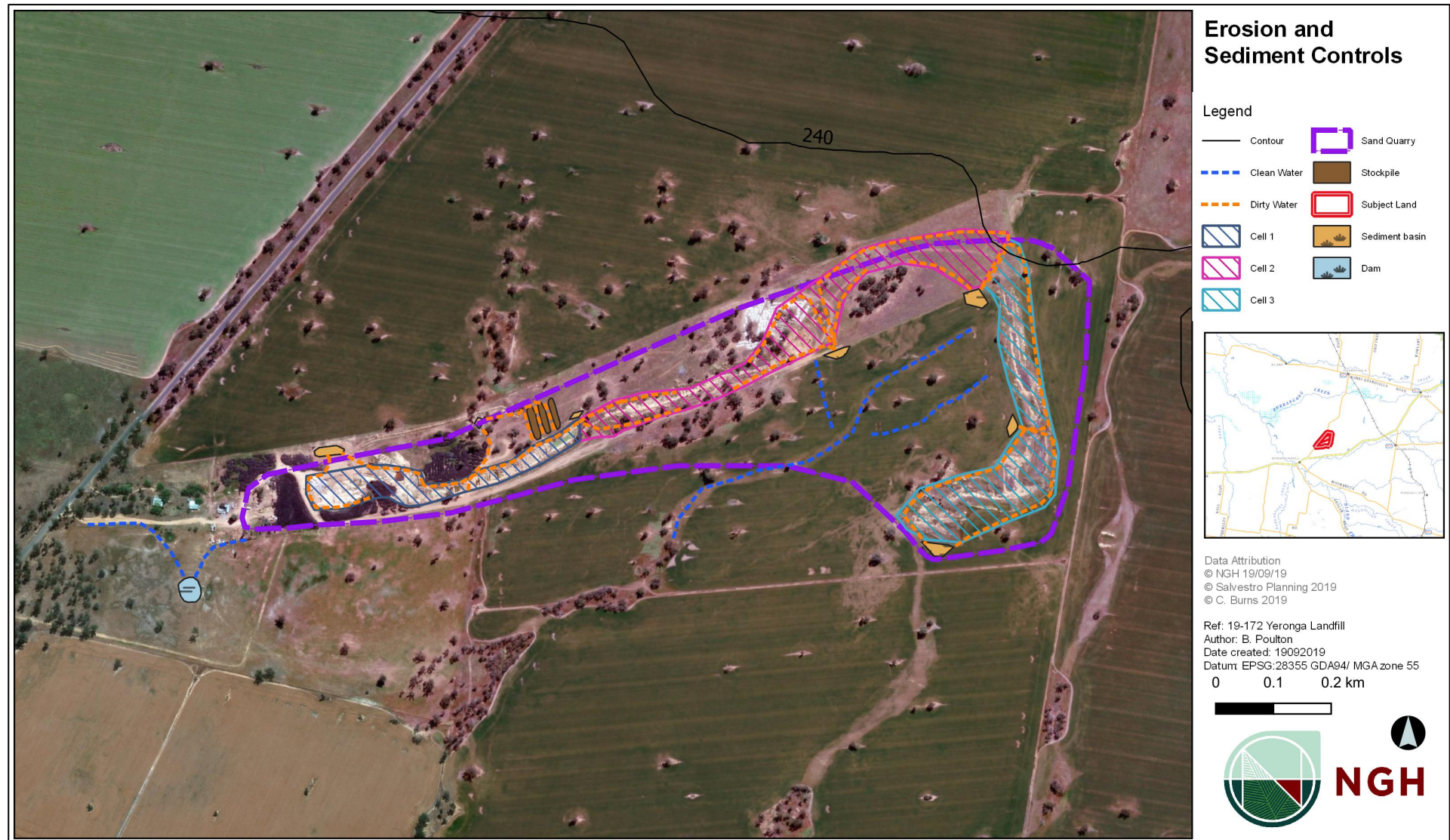
Figure 6-1 Erosion and sediment controls
